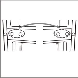
9. Unscrew bottom hinge. Then remove the adjustable feet from both side.
