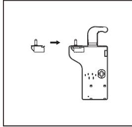
5. Detach cover in top of upper door and move harness from right side to left side, then replace the cover.
