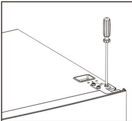
3. Remove the pin with a screwdriver and flip the hinge bracket. Then refit the pin to hinge bracket
