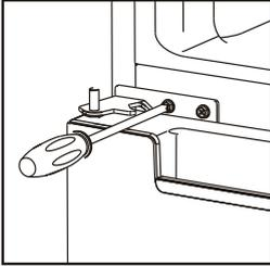
15. Replace upper door, please ensure the door align with the cabinet to make sure door gasket seal the cabinet tightly. Then connect door with cabinet by tightly fixed top hinge.
