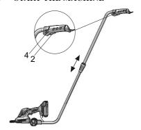
Press the lock-off button (4) and hold while actuating the on/off switch (2).
