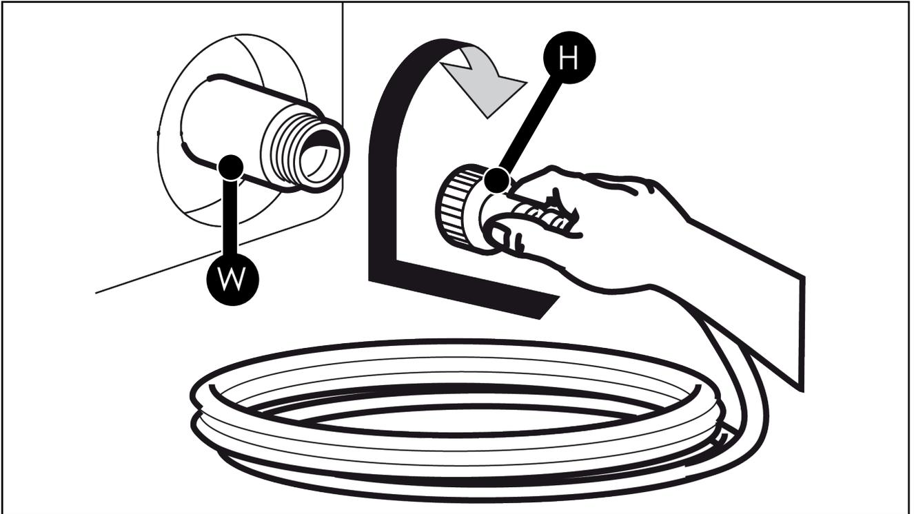
2. Attach the high pressure hose (H) to the gun (G), it will click into place. To release the high pressure hose, push the release button (Z1). If the trigger is not depressed whilst disconnecting the lance from the hose, the connector may be hydro-locked and it will not be possible to remove. Excess pressure that can occur even after the unit is shut down can be released by squeezing the trigger.
