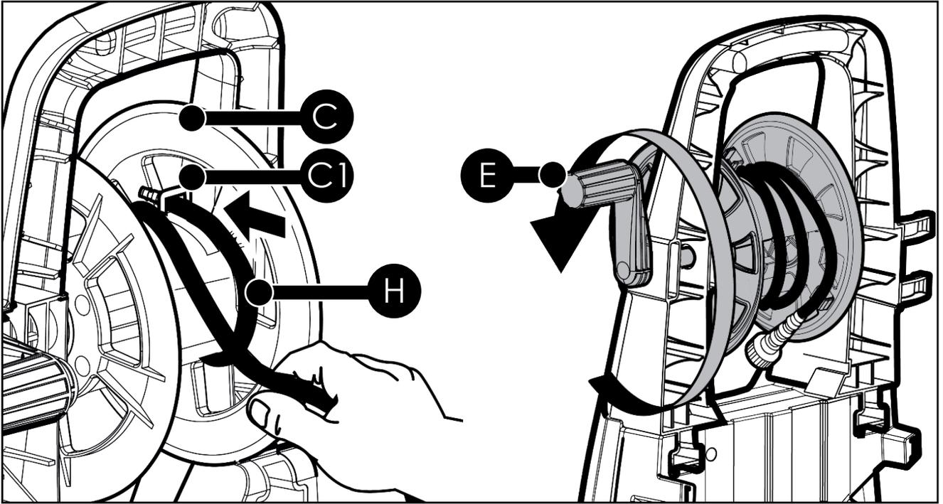
8. When winding the hose storage reel, make sure it is tidy and not overlapping at all.
