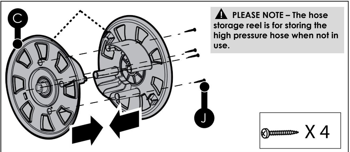
2. Push the hose storage reel (C) into place on the carry handle (B).
